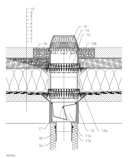
TO HEAT THE DRAIN, YOU MAY USE HEATING KIT HL609 WITH SELF-REGULATING HEAT SOURCE 36W/23OV. (THE HEATING TAPE MUST BE WRAPPED AROUND THE DRAIN BODY BEFORE INSTALLATION).
