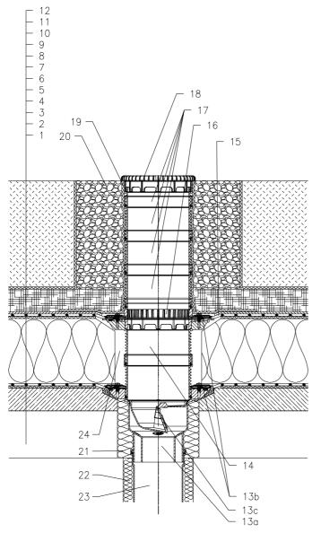
TO HEAT THE DRAIN, YOU MAY USE HEATING KIT HKL156 WITH REGULATING HEAT SOURCE 40W/M; 230 V; (APR. 12-14W HEATING TAPE). (THE HEATING TAPE INCL. THERMAL INSULATION MUST BE PULLED ON THE DRAIN BODY BEFORE INSTALLATION) RECOMMENDED BOREHOLE DIAMETER IS @220mm, 22020x20mm. DURING INSTALLATION TAKE CARE, THAT THE FLANGE POSITION IS ON THE LOWEST LEVEL OF DRAINAGE. WE RECOMMEND, TO SITE IT APPR. 1cm BELOW THE SCREED. TO AVOID CONDENSATE WATER TAKE CARE OF THERMAL INSULATION ON THE CONSTRUCTION SITE.
