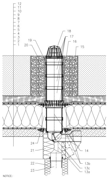
TO HEAT THE DRAIN, YOU MAY USE HEATING KIT HL82 WITH SELF-REGULATING HEAT SOURCE 18W/22OV. (THE HEATING TAPE MUST BE WRAPPED AROUND THE DRAIN BODY BEFORE INSTALLATION).
