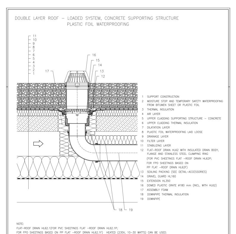
ASSEMBLY INLET: ø255 mm, OR 255 x 380 mm
