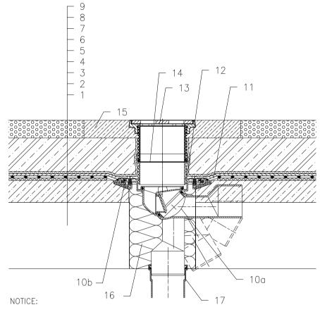
TO HEAT THE DRAIN, YOU MAY USE HEATING KIT HL82 WITH SELF-REGULATING HEAT SOURCE 18W/22OV. (THE HEATING TAPE MUST BE WRAPPED AROUND THE DRAIN BODY BEFORE INSTALLATION).
